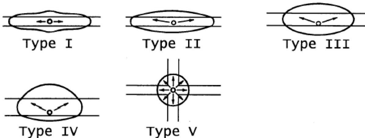
In addition to these types, the light distribution can also be classified as short, medium, or long. This refers to the luminaire's vertical light distribution and is based on where the maximum intensity (candela value) points to in relation to the luminaire pole.
