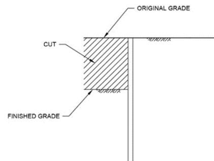
*Pile Retaining Wall Section as an Example of Cut Construction*
