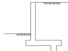
*Cantilever Retaining Wall Section as an Example of an Externally Stabilized Wall*
