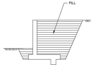
*Cantilever Retaining Wall Section as an Example of Fill Construction*
