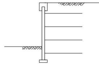
*MSE Wall Section as an Example of an Internally Stabilized Wall*
